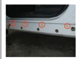
6. Peal off the covers to reveal the threaded holes in the sill (5 in total).
