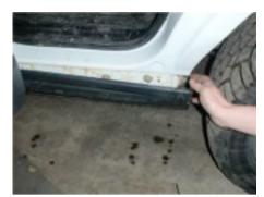
5. Remove the 9 plastic clips from the sill.
