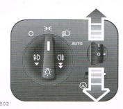
With the headlamps turned on, rotate the thumbnail up or down to adjust the vertical aim of the beams.
