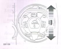
You will need to gain access to the inside of the headlamp unit. See REMOVING A HEADLAMP (page 93). Move the lever down for when driving in left-hand drive countries and up for right-hand drive countries.
