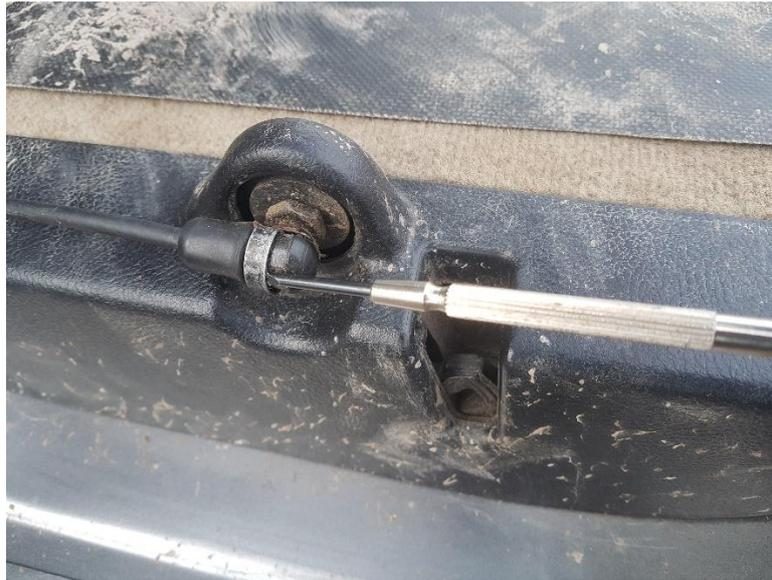
Next, remove the hinged panel flap that extends across the boot over the hinges of the tailgate.
