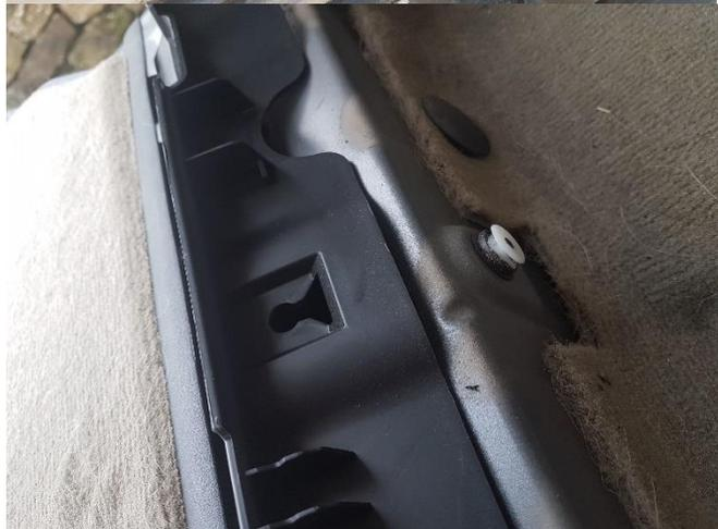
Next, remove the two spring loaded luggage loops on the floor of the boot, one Hex socket (Allen key) bolt each, as these hold down the carpeted trim next to the side trim which holds it in place.
