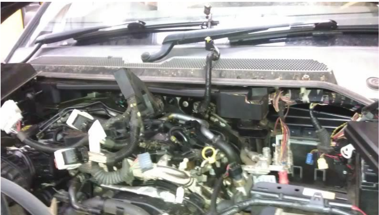
Glow plug wiring stays with the body
