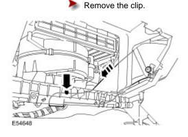
Remove the passenger side footwell duct elbow.
