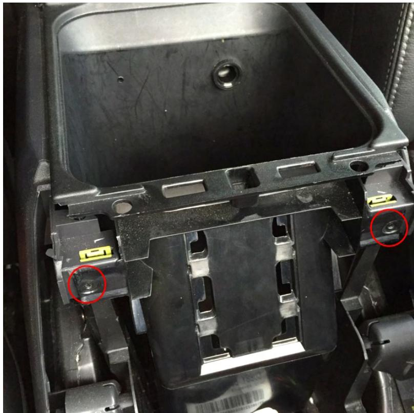
Grip either side of the cubby box and pull firmly upwards. It needs quite a pull! You now have access to the back of the rear vent panel.
