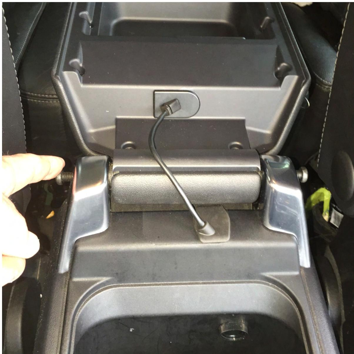
Pull off the two plastic covers and pull the lid hinge upwards to separate it. Put it to one side but be careful not to stretch the USB lead if fitted.
