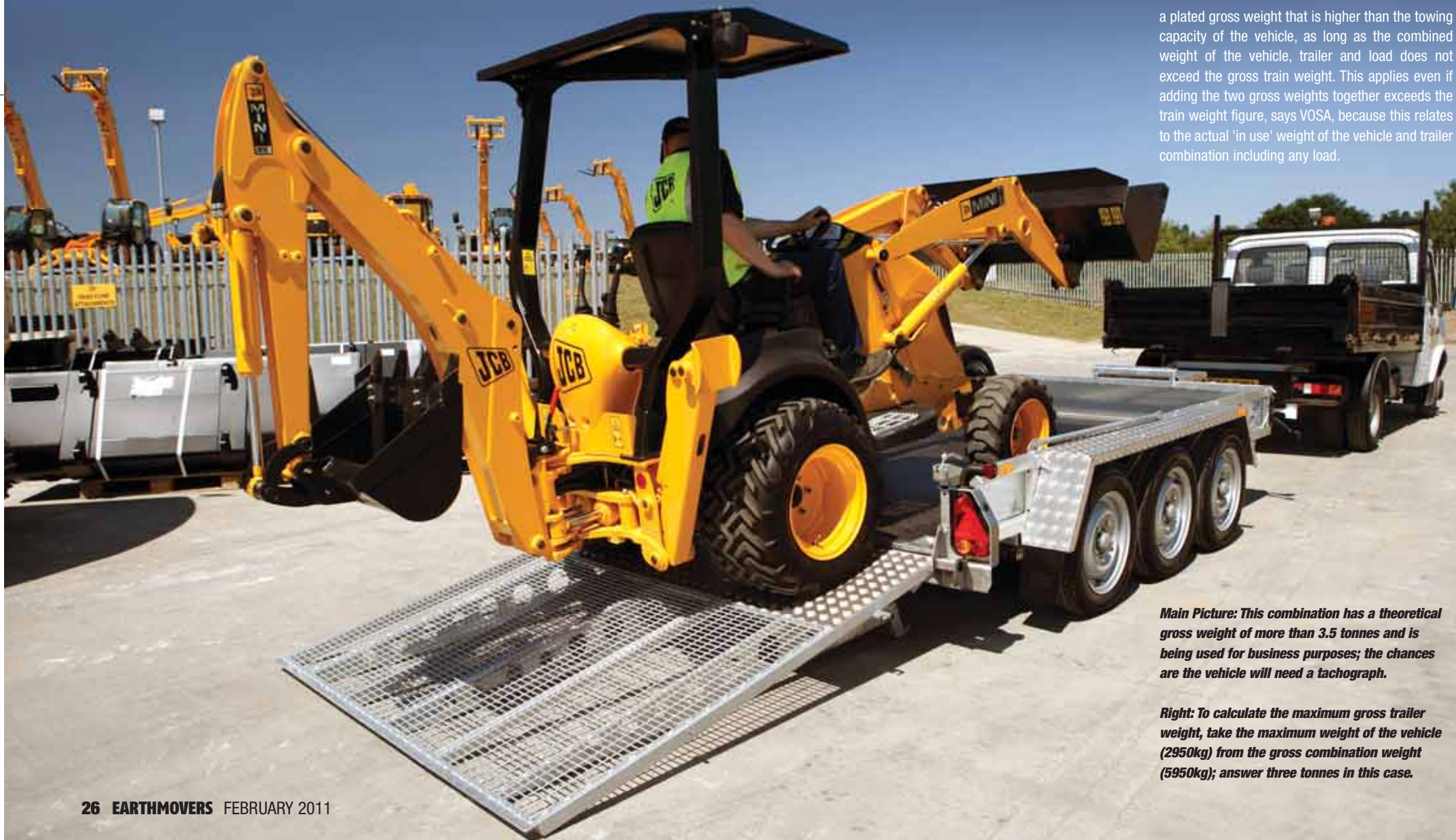
Above: With a decent sized mini on board, the gross weight of this trailer is approaching 3.5 tonnes. Towing it with a vehicle lighter than this will require a careful risk assessment.
