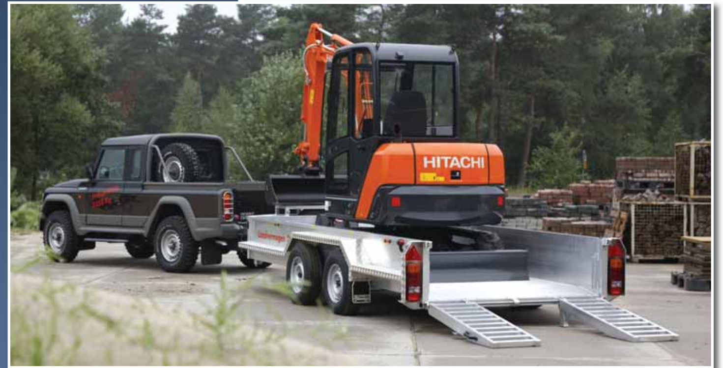
Above: With a decent sized mini on board, the gross weight of this trailer is approaching 3.5 tonnes. Towing it with a vehicle lighter than this will require a careful risk assessment.
