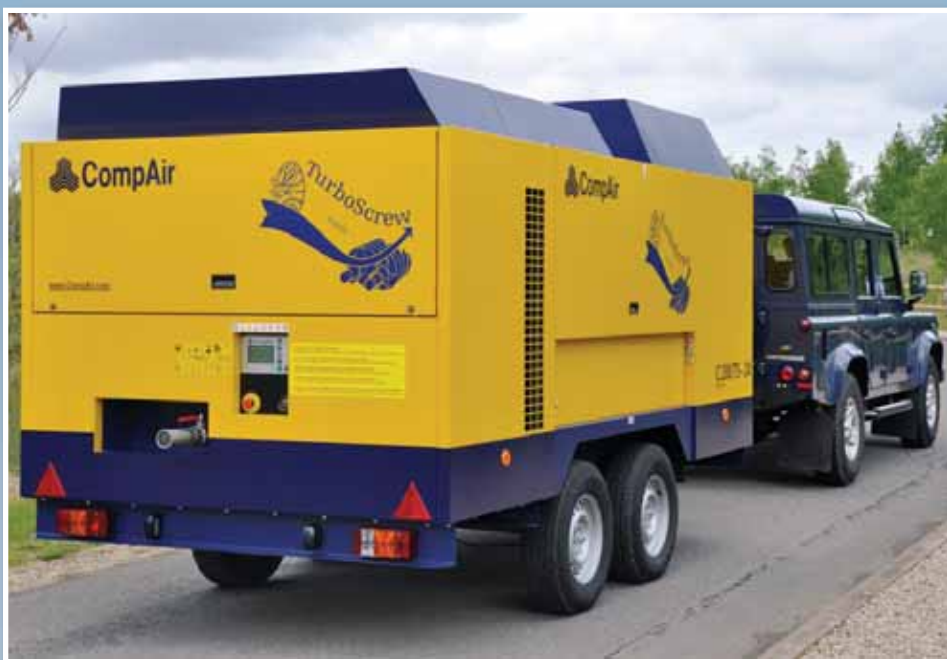
Left: This trailer weighs nearly 3.5 tonnes, which probably means that an O-licence is required to be held by the enterprise that tows it on the road.
